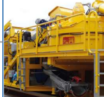
Mescolatore planetario MEP 1500 - 1,5 m 3 resa Planetary mixer MEP 1500 - 1,5 m 3 capacity
