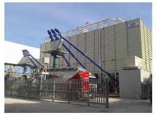
Screw conveyors are strongly recommended in low level installations because they help to maintain the whole setup within specific limits, which can be set by permitting authorities.
